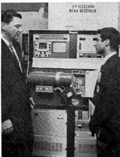
3M Co.'s electron beam recorder development for making 16mm film prints directly from video tape masters is described by Jerrold A. Friedman (r), chief engineer, WVBR-FM Ithaca, N.Y., by John Reeds of 3M Co.
